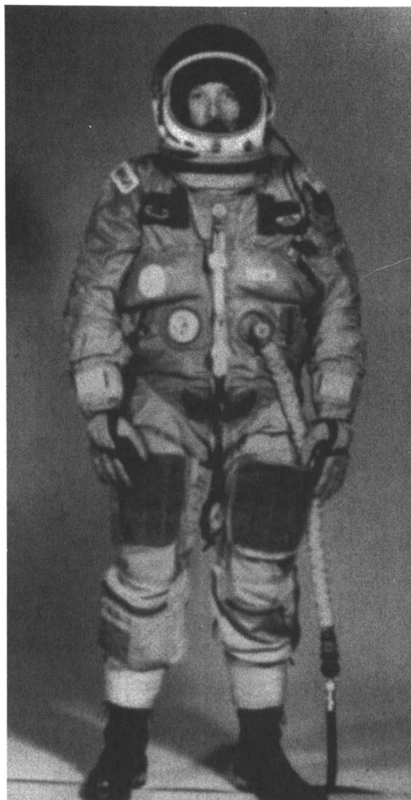
Figure 11. Astronaut's polybenzimidazole (PBI) lift-off suit
